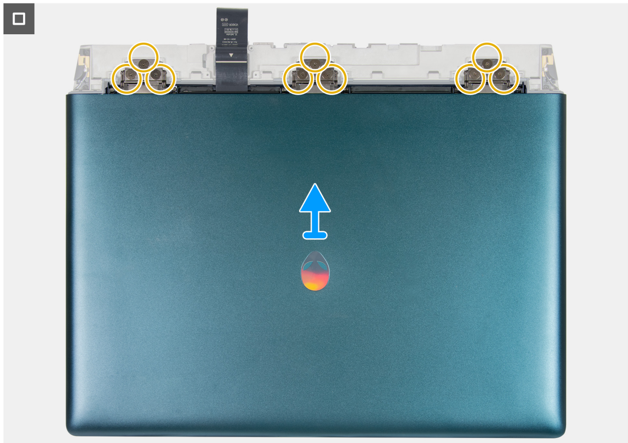
Figure 52. Removing the display assembly
