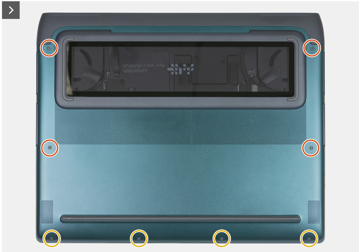
Figure 10. Removing the base cover screws
