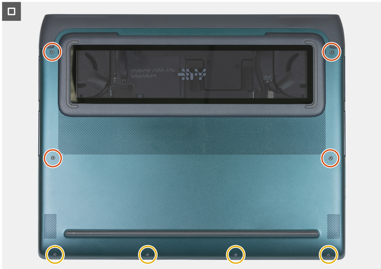
Figure 15. Replace the base cover screws
